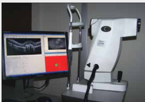
Figure 2. Bioptigen SDOCT clinical scanner and software interface, showing retinal B-scan, en face image, and fixation target.
